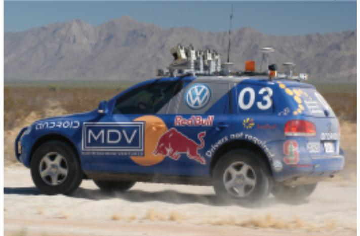
Sebastian Thrun headed up a team of five who mounted on the VW's rooftop a GPS system, a laser range-finder that can look 30 meters ahead while scanning side to side, and a video camera that sends data back from down the road so the car can see 80 meters ahead. Photo sensors in a wheel well monitor how far the car has traveled.
