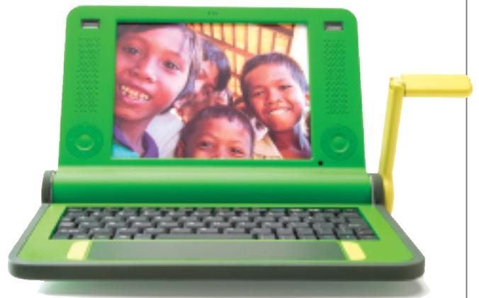
area networks through mesh networks. The power source was a crank-operated generator, but several exterior generators are being tested. The cases are tough plastic that seal shut to keep out rain and dust as kids take them to and from school.
